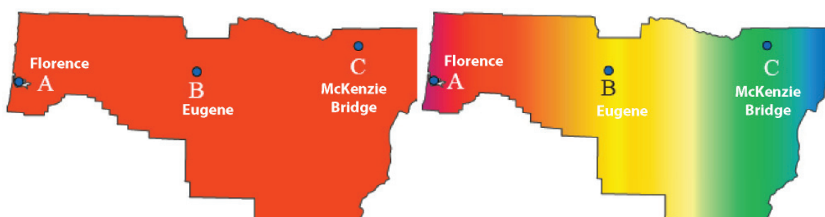
Figure 1. Variation in assigned seismic hazard level within Lane County, Oregon. (left) The RVS seismicity classification by county system assigns the entire county the same classification on the basis of the the highest seismicity location. (right) schematic of real variation of seismic hazard levels, with the seismic hazard decreasing markedly from west (red) to east (blue).
